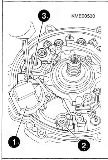
ASSEMBLING ALTERNATOR Assembling regulator Fasten connection/terminal V (1). Use torque wrench. Tightening torque Terminal V: 1,0...1,4 Nm Torque wrench: comm. avail. comm. avail.
